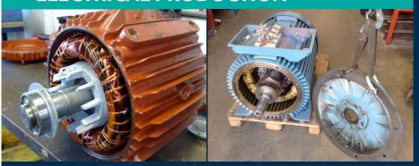
Available equipment ensures performance of electrical, adjustment–alignment and repair works on the units, which are under construction and repair, allows the rewinding of stators and rotors of electrical machines of up to 0,5 MW.
